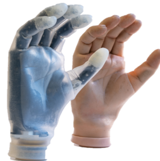
SoftHand Pro prosthesis with cosmetic glove
